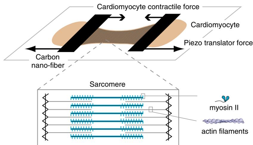
**Fig. 5** Single cardiomyocyte dynamic force–length measurements: cartoon schematic of a cardiomyocyte (light brown) suspended between two carbon nanofibers. The carbon nanofibers act as calibrated force transducers, whose displacement is a dynamic readout of the force generated by the cardiomyocyte. The carbon nanofibers can be coupled to a piezo-translator. This provides a high-frequency feedback that adjusts the position of the carbon nanofiber during
