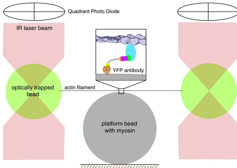
**Fig. 4** Optical trapping of myosin molecules: cartoon schematic of a dual-beam laser optical trap for measuring the lever-arm stroke, force generation, and kinetics of single myosin molecules. Streptavidin-coated polystyrene beads are optically trapped by a focused infrared (IR) laser beam. An optically trapped bead is attached to each end of a single biotinylated actin filament (*gray line*). The filament is stretched using fluorescently labeled phalloidin. The actin filament is stretched
